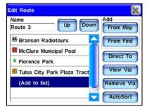
Use the Routes list menu (left) to store and manage different routes. The Edit Route screen, at right, shows the details of a stored route. Each route contains different "legs." Each leg is a destination in the route. The Edit Route screen contains all of the routing controls for a generated route from the Routes list.
